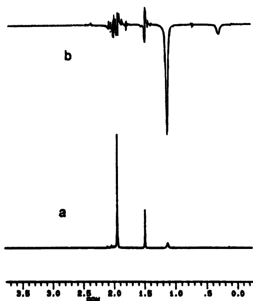
Fig. 1. (a) ^1\text{H} NMR spectra of A at 223 K. (b) Difference spectrum of A at 223 K with irradiation of the \mu\text{-Ti-Me} resonance at \delta 1.12.
